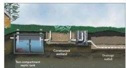
Figure 2.7 Constructed Wetland System
