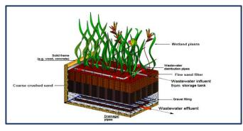
Figure 2.8. Horizontal flow constructed wasteland design. Adopted from Napaldet, J. & Buot, I. (2019).
