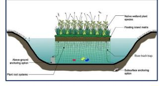
*Figure 2.9.* Schematic diagram of constructed floating wetland adopted from Tanner, C. et. al. (2011)
