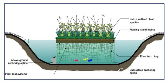
Figure 2.17. Schematic diagram of constructed floating wetland adopted from Tanner, C. et. al. (2011)
