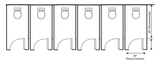
Figure 2.5 Floor Plan of the Centralized Toilet Room with Six Cubicles
