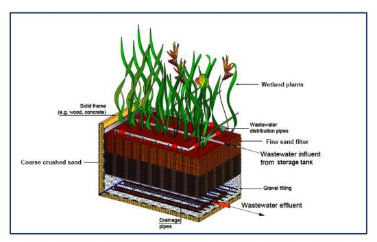
Figure 2.13. Horizontal flow constructed wasteland design. Adopted from Napaldet, J. & Buot, I. (2019).
